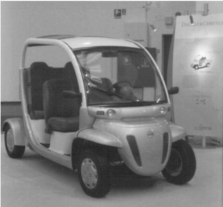
Figure 11.3 An example of the low speed vehicle (LSV) type of electric car
