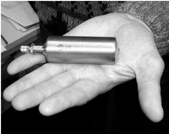
Figure 5.5 Metal hydride stores can be made quite small, as this example shows
