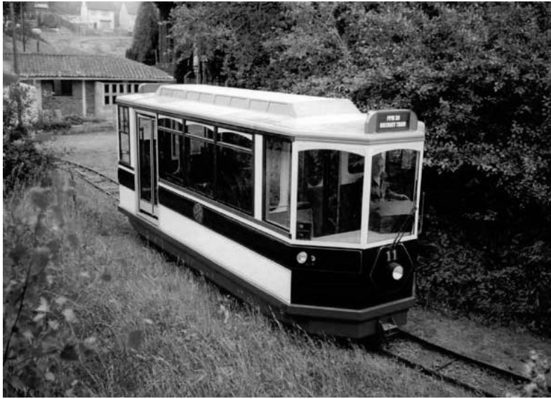
Figure 1.17 The Parry People Mover. This electric vehicle uses a flywheel to store energy (Photograph kindly supplied by Parry People Movers Ltd.)
